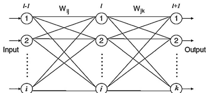
Fig. 1. Three-layer feed-forward ANN architecture.
